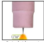
Optimal stickout varies by electrode type and diameter but is usually approximately 1/16"
